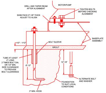
After the grout has cured and you have tightened the foundation bolts, you must check the alignment of the pump and driver.
