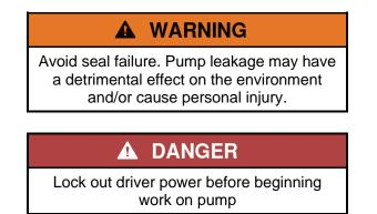
Refer to the seal manufacturer's installation, operating, and maintenance instructions. Failure to do so can result in environmental damage, personal injury, and seal malfunction and/or seal failure. Pay particular attention to paragraphs 4.2, 4.3 and 4.4.
