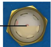
Figure 5-1: Proper Oil Level
