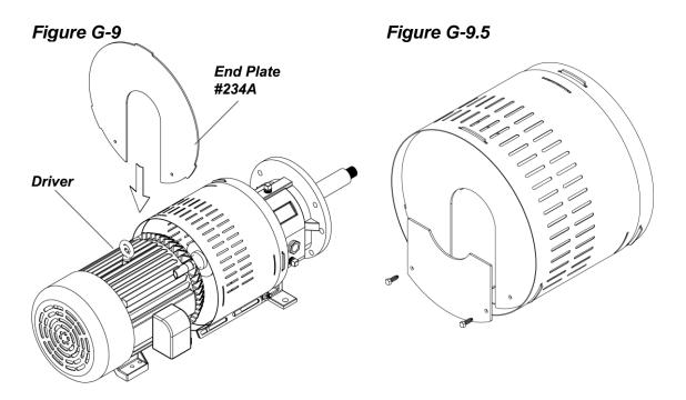
6. Adjust the length of the coupling guard to completely cover the shafts and coupling as shown in *Figure G-10,* by sliding the coupling guard half (driver end) toward the motor. After adjusting the length, secure the guard with a bolt, nut and two (2) washers through the slotted holes at the center of the guard and tighten. Check
