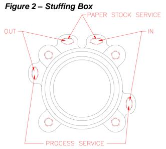
There are four pipe taps on the standard stuffing box cover. (See *Figure 2*.) Two are alternately used as in and out connections for process / chemical services and the other two are used for in and out connections for paper stock service.
